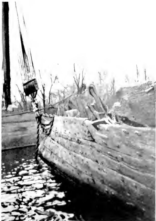
STERN-QUARTER OF THE "JUGOSLAVIJA" WITH THE PARTS OF THE ASHES OF HER PLANKING WHERE THE ACID WAS KEPT - IN THE FOREGROUND THE COAL
